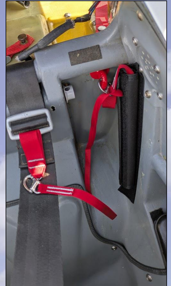
Style #2 - Static Line container mounted onto the glider
