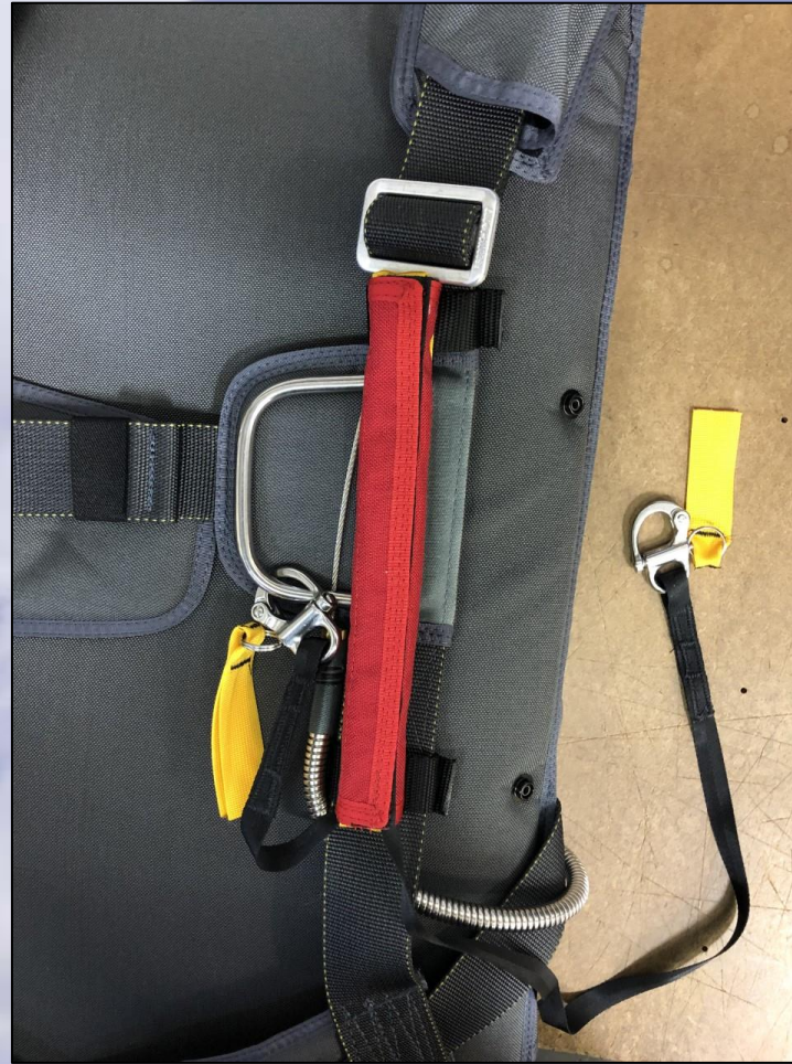
Style #1 - Static Line container mounted onto the parachute
